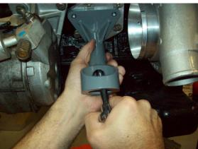
Snug the bolt so it allows some movement to align the remaining bolt holes. Install the remaining 20mm and one 35mm (USDM Passenger side only) bolts with washers and torque all three per side to 35 ft-lbs (47 N-m).
