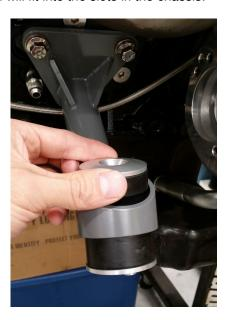
Place the thinner upper bushing with its aluminum washer onto the top of the mount and install the M10 x 70mm long flat head bolt – it is very critical that you use grease on these particular bolts, since the bolts thread directly into aluminum.
